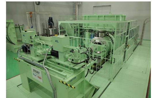
風力発電機用ベアリング専用試験機 Special test equipment for the large bearings used in large bearings
